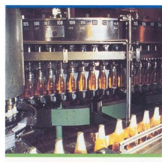
THE MILLER BREWING COMPANY USES A CONTINUOUS PRODUCTION PROCESS. BEER IS BREWED, BOTTLED, PACKAGED, AND SHIPPED ON ONE LONG PRODUCTION LINE WITH SPECIALIZED AUTOMATED EQUIPMENT.
