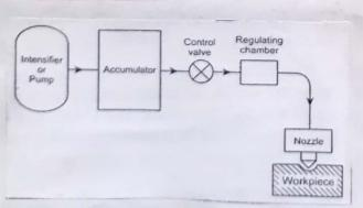
Fig: Schematic diagram of WJM
