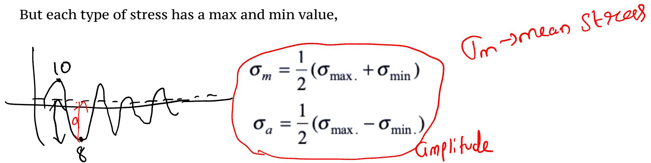
It can be observed that repeated stress and reversed stress are special cases of fluctuating stress
