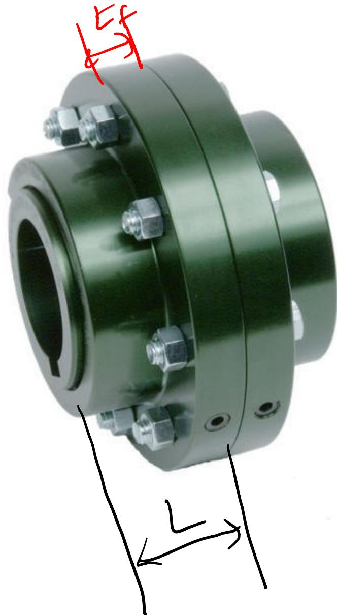
**Unprotected type flange coupling.** In an unprotected type flange coupling, as shown in Fig, each shaft is keyed to the boss of a flange with a counter sunk key and the flanges are coupled together by means of bolts.
