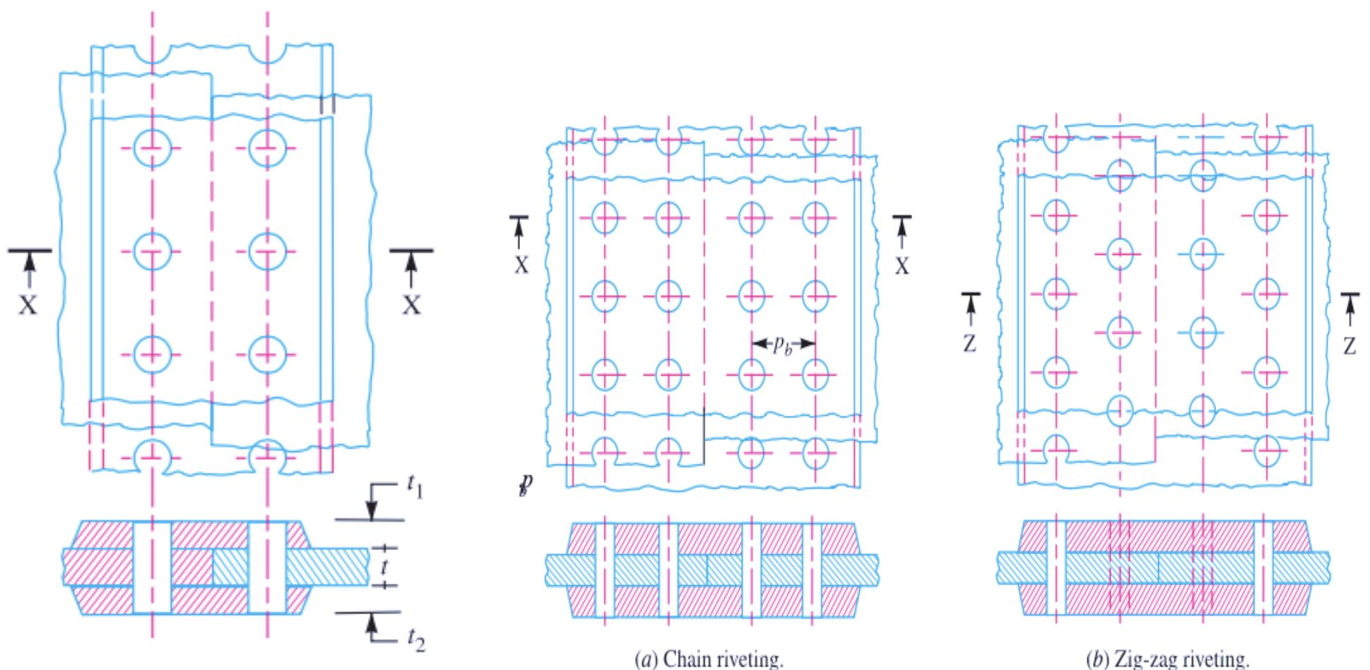
**Fig. 9.8.** Single riveted double strap butt joint.
