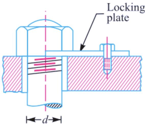
**Fig. 11.20.** Locking with plate.
