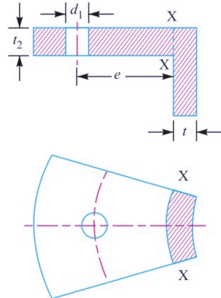
**Fig. 11.26.** A portion of the cylinder flange.
