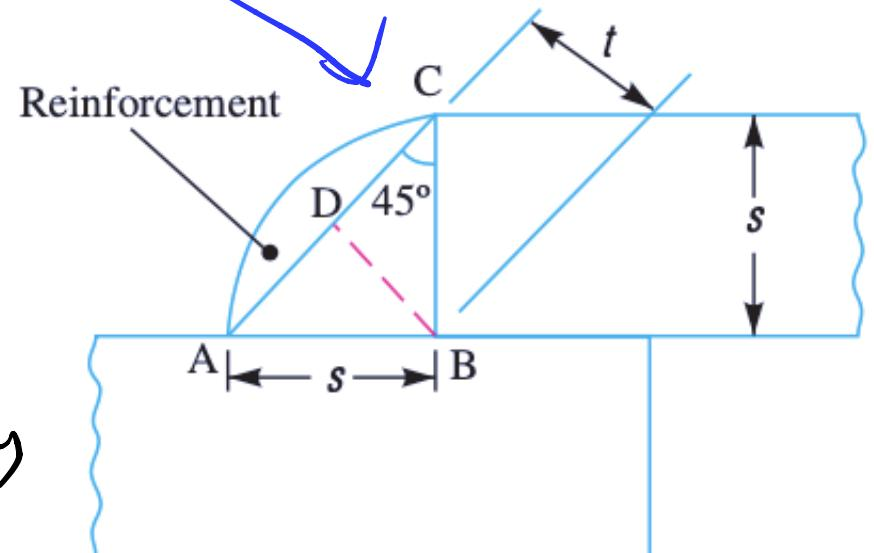
Fig. 10.7. Enlarged view of a fillet weld.
