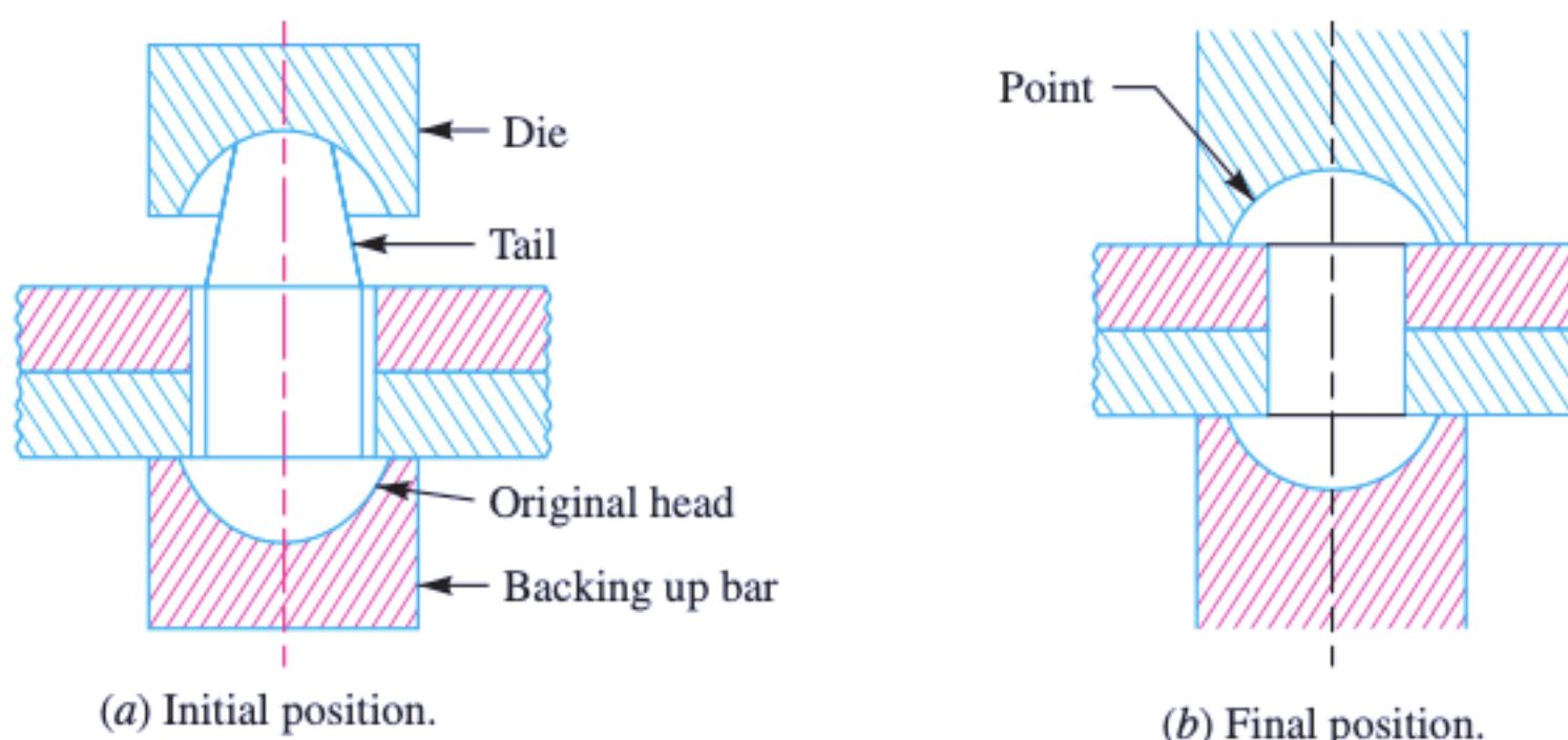
A cold rivet or a red hot rivet is introduced into the plates and the *point* (i.e. second head) is then formed. When a cold rivet is used, the process is known as *cold riveting* and when a hot rivet is used, the process is known as *hot riveting*. The cold riveting process is used for structural joints while hot riveting is used to make leak proof joints.
