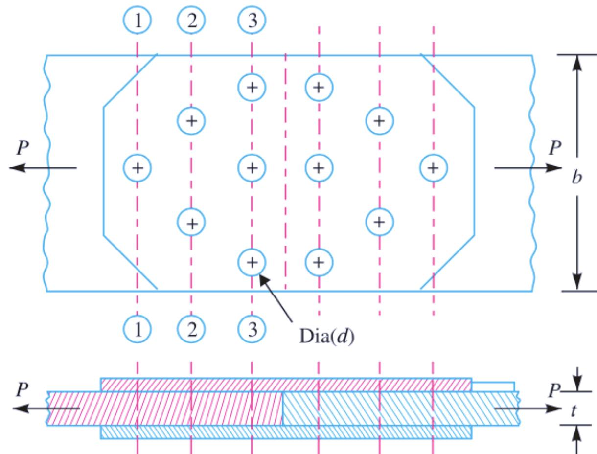
**Fig. 9.19.** Riveted joint for structural use.
