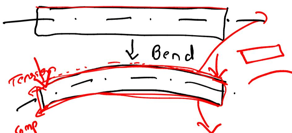
Combination of tensile, comp & shear stress.
