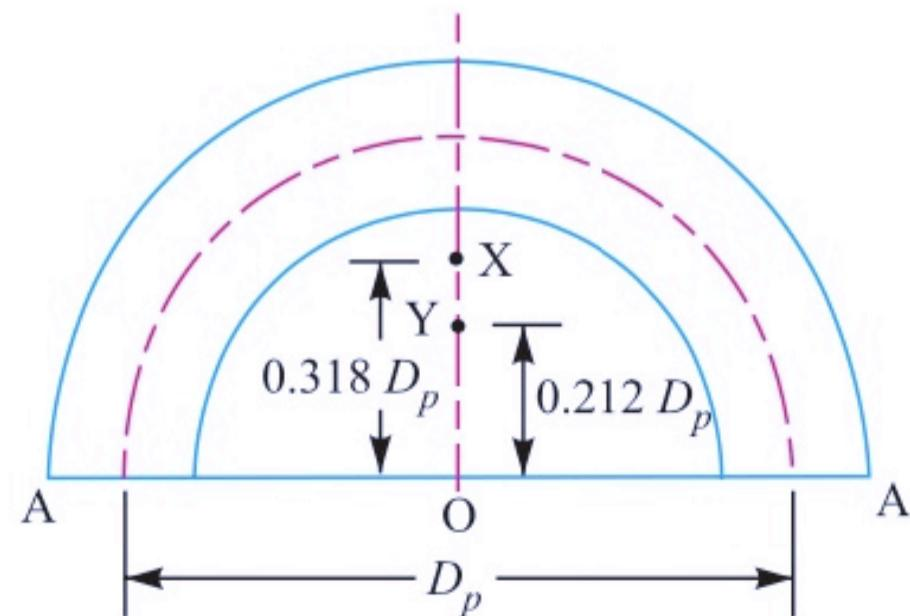
Fig. 11.25. Semi-cover plate of a cylinder.
