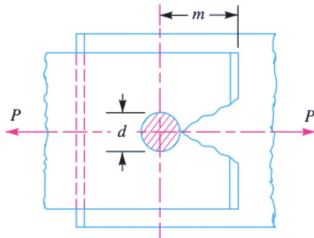
Fig. 9.13. Tearing of the plate at an edge.
