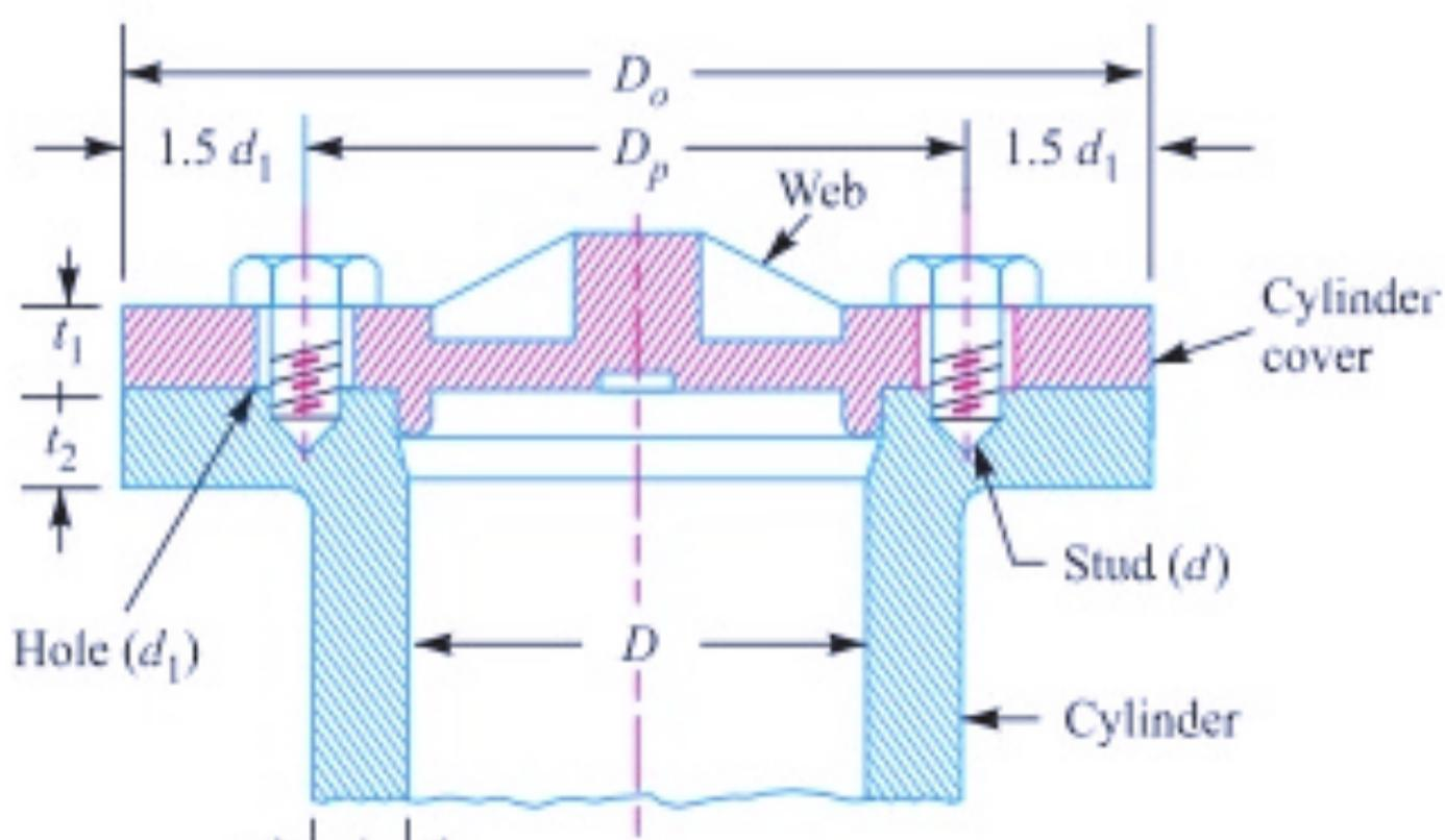
(b) Arrangement of securing the cylinder cover with studs.
