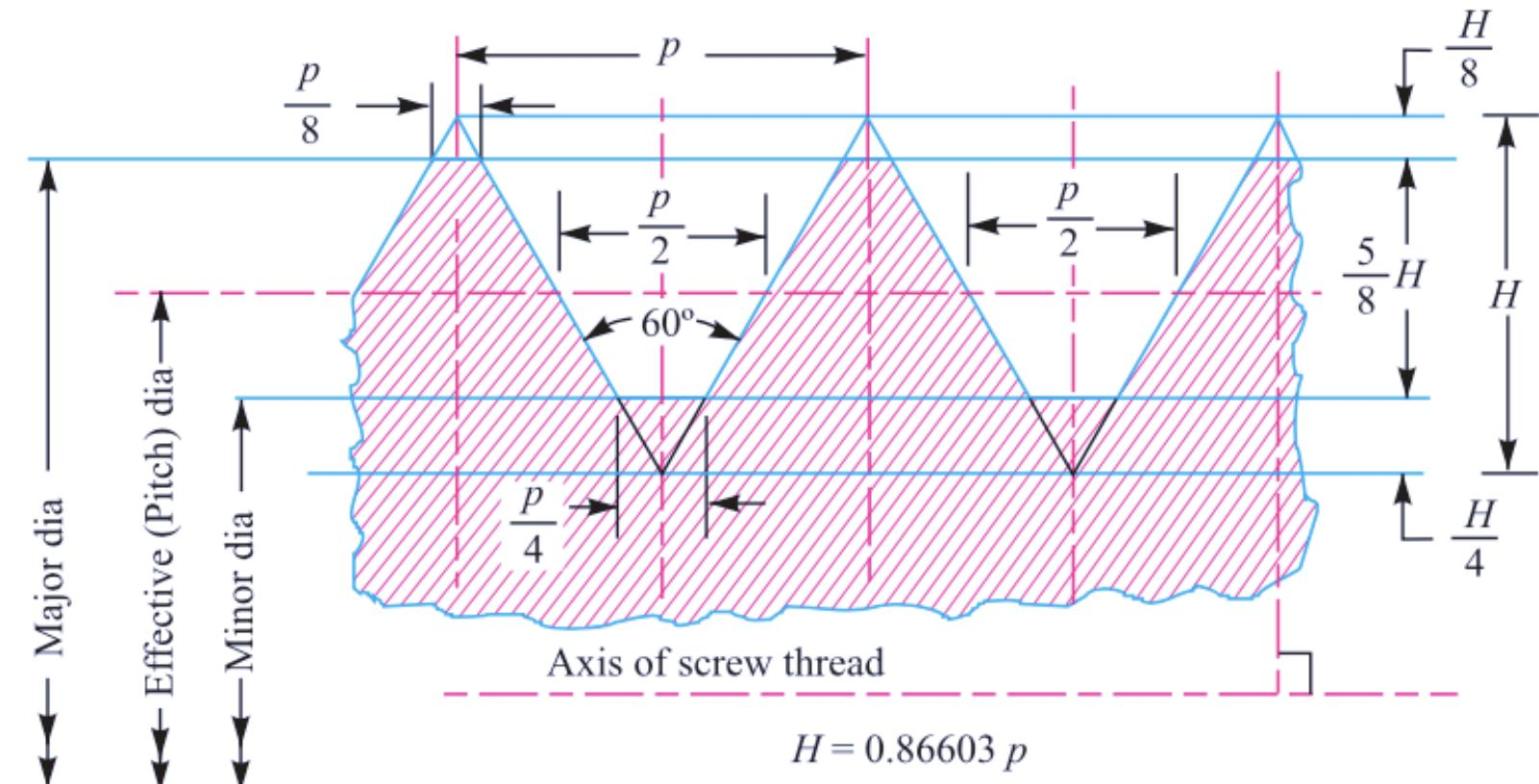
**Fig. 11.10.** Basic profile of the thread.
