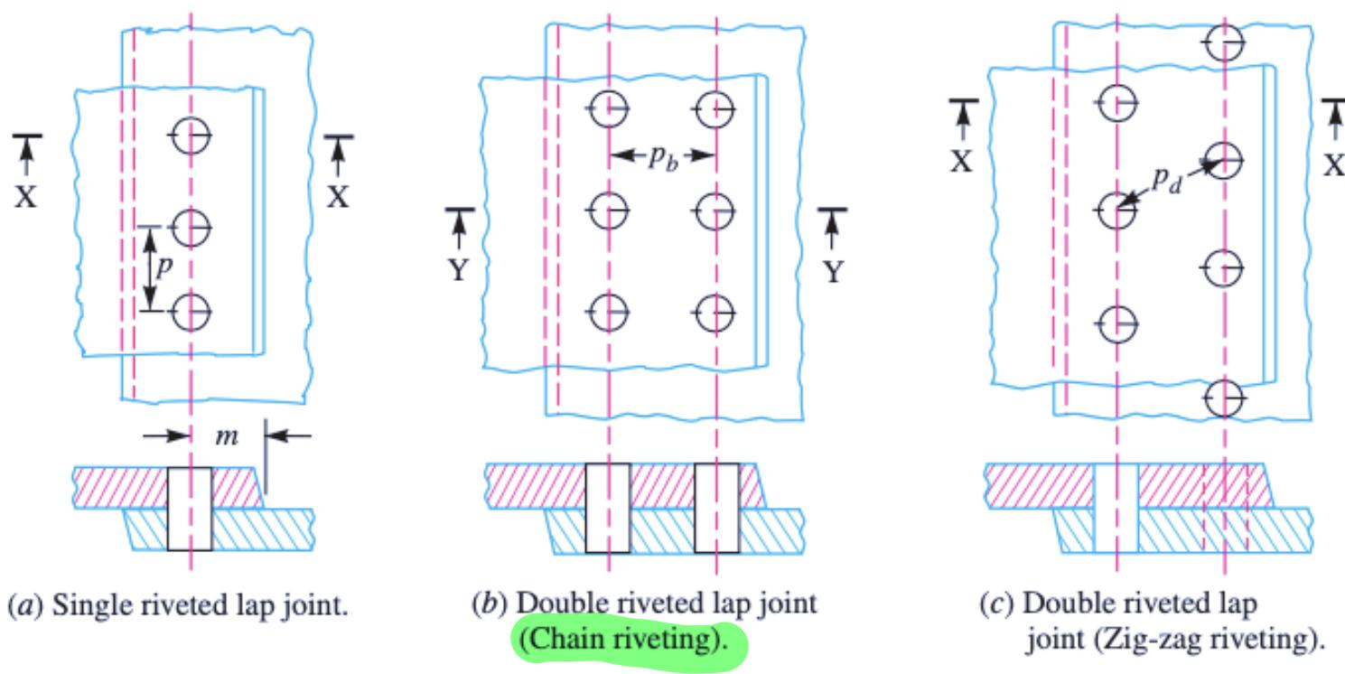
**Fig. 9.6.** Single and double riveted lap joints.
