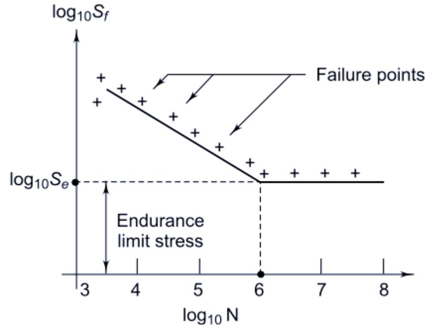
Fig. 5.20 S-N Curve for Steels
