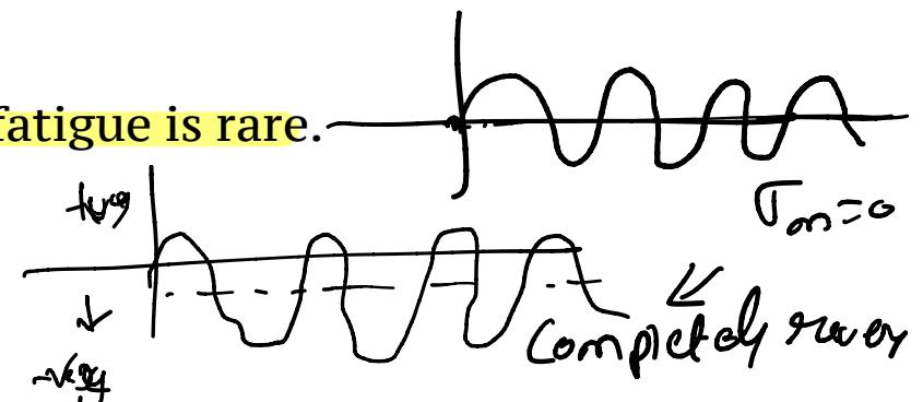
The point  $\sigma_e$  represents the fatigue strength corresponding to the case of complete reversal ( $\sigma_m = 0$ ) and the point  $\sigma_u$  represents the static ultimate strength corresponding to  $\sigma_a = 0$ .
