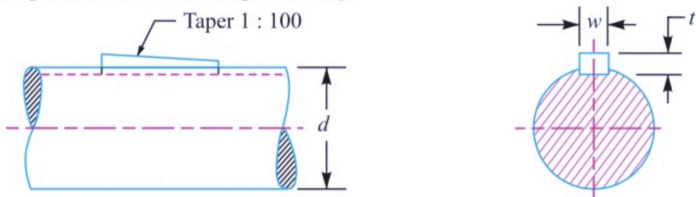
**2. Square sunk key.** The only difference between a rectangular sunk key and a square sunk key is that its width and thickness are equal, i.e.
