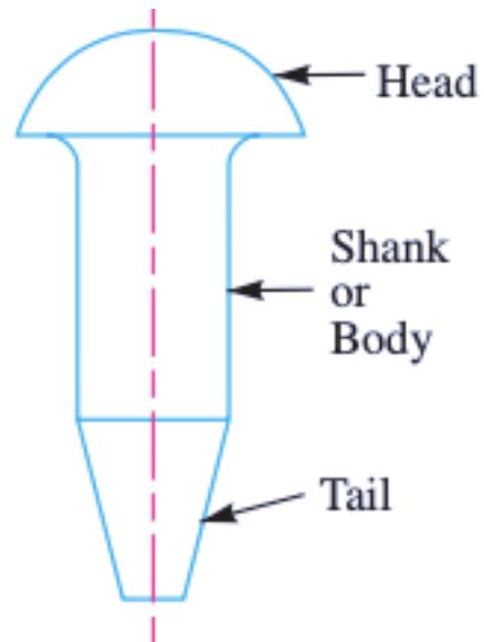
The rivets are used to make permanent fastening between the plates such as in structural work, ship building, bridges, tanks and boiler shells. The riveted joints are widely used for joining light metals.
