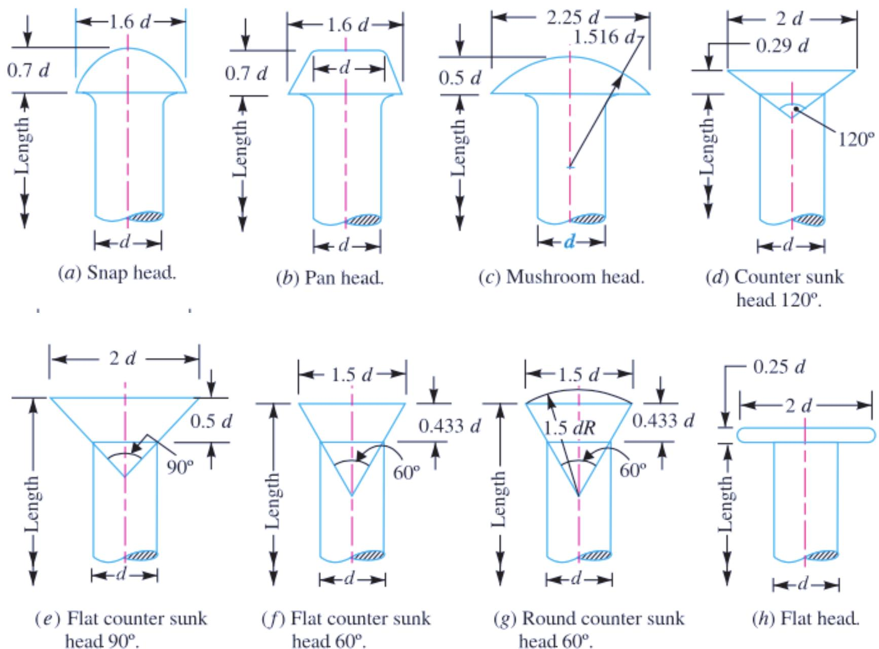
The **snap heads** are usually employed for structural work and machine riveting.
