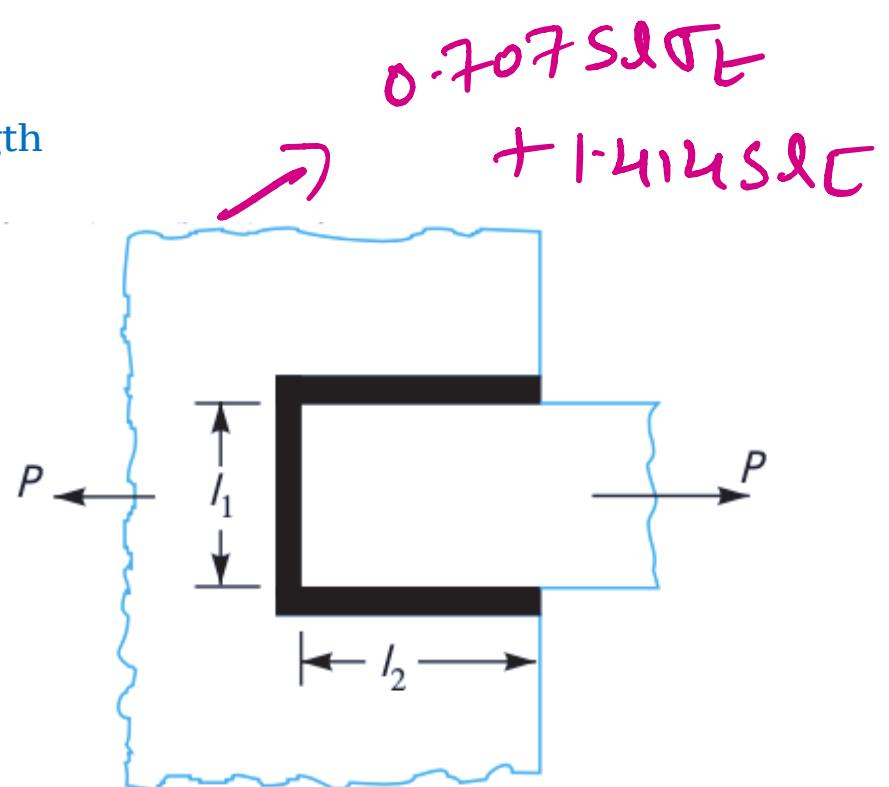
(b) Combination of transverse and parallel fillet weld.
