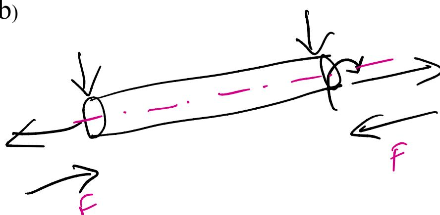
$$\frac{M}{I} = \frac{\sigma_b}{y} \quad \text{or} \quad \sigma_b = \frac{M \cdot y}{I} = \frac{M \times d/2}{\frac{\pi}{64} \times d^4} = \frac{32M}{\pi d^3}$$
