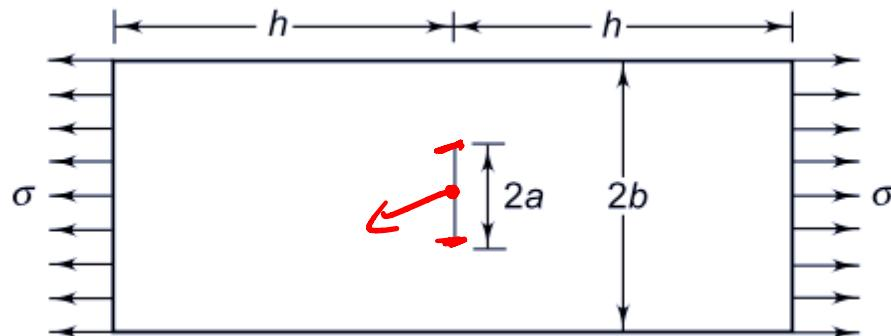
The stress intensity factor  $K_0$  specifies the stress intensity at the tip of the crack.
