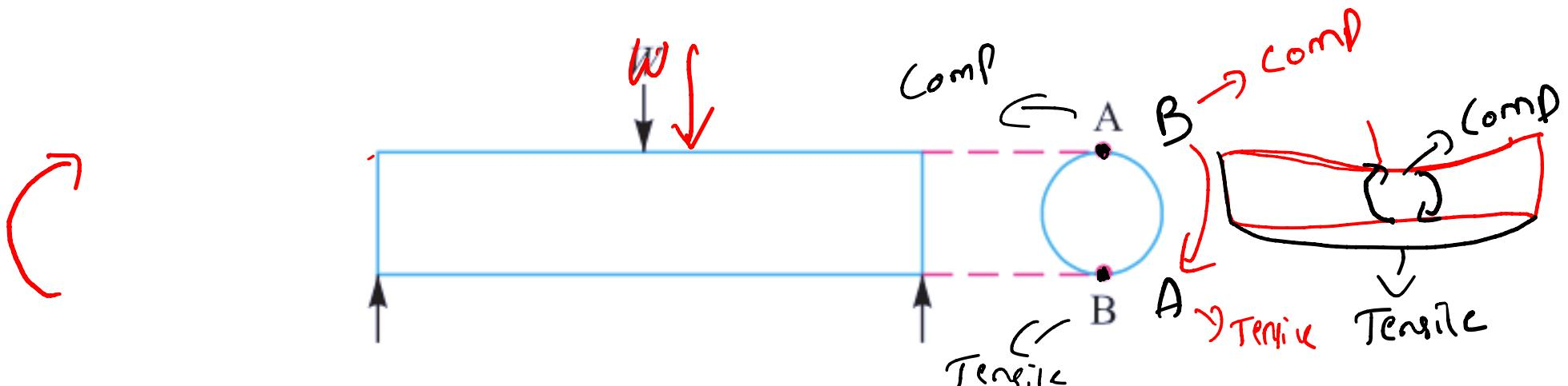
Upper fibres of the beam (i.e. at point A) are under compressive stress and the lower fibres (i.e. at point B) are under tensile stress
