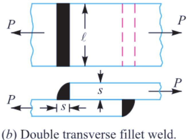
The transverse fillet welds are designed for tensile strength
