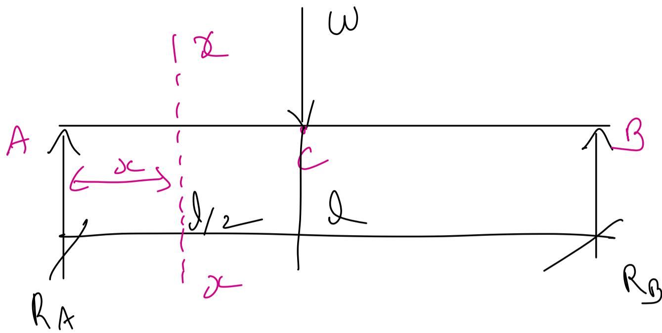
$$R_A + R_B = \omega - (1) \quad \text{B.M @ Point A} = 0$$
