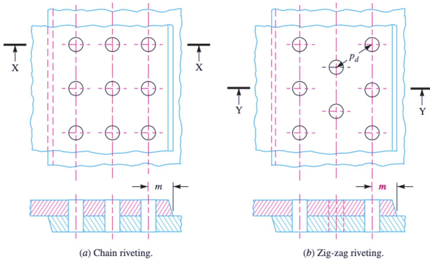
**Fig. 9.7.** Triple riveted lap joint.
