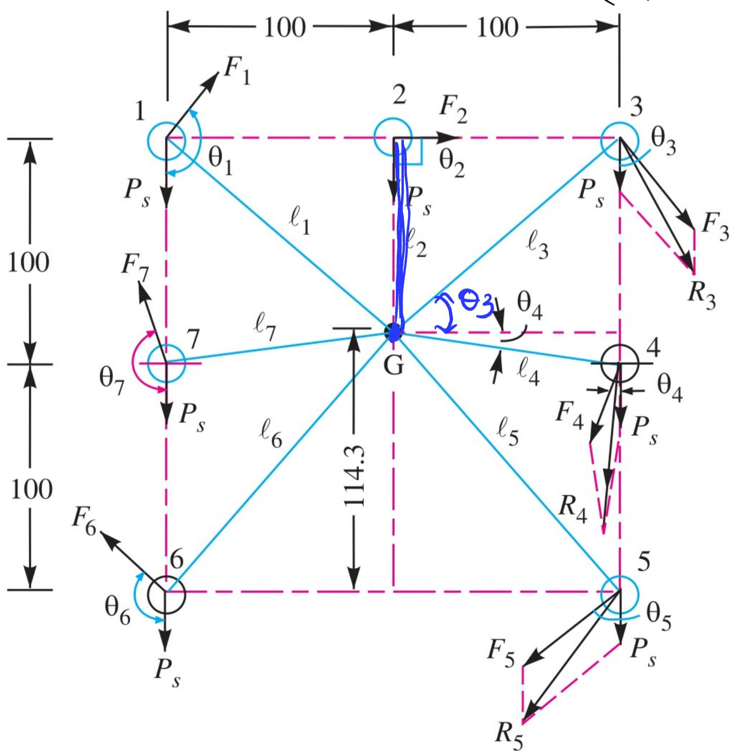
$$P_{xe} = F_1 l_1 + \bar{F}_2 l_2 + \bar{F}_3 l_3 + \bar{F}_4 l_4 + F_5 l_5 + \bar{F}_6 l_6 + \bar{F}_7 l_7$$
