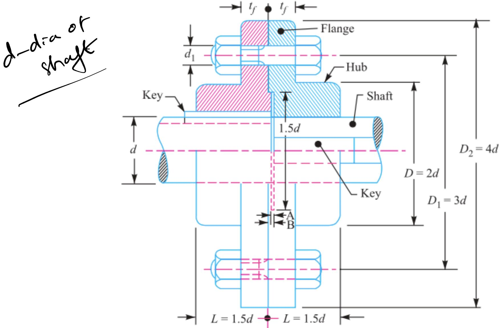
If  $d$  is the diameter of the shaft or inner diameter of the hub, then
