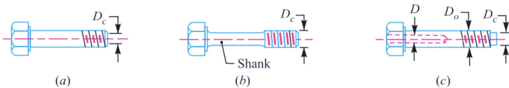
A second alternative method of obtaining the bolts of uniform strength is shown in Fig (c). In this method, an axial hole is drilled through the head as far as the thread portion such that the area of the shank becomes equal to the root area of the thread.
