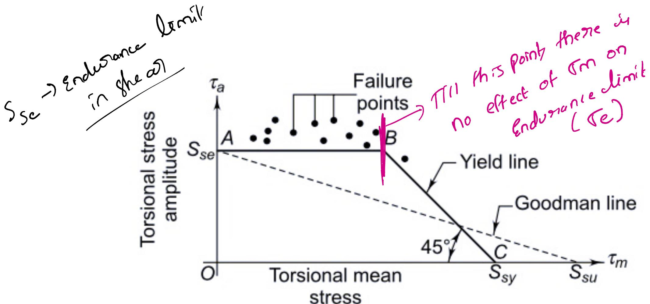
**Fig. 5.41** Modified Goodman Diagram for Torsional Shear Stresses
