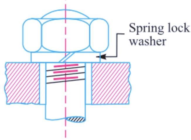
**Fig. 11.21.** Locking with washer.
