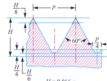
Fig. 11.5. Unified standard thread.
