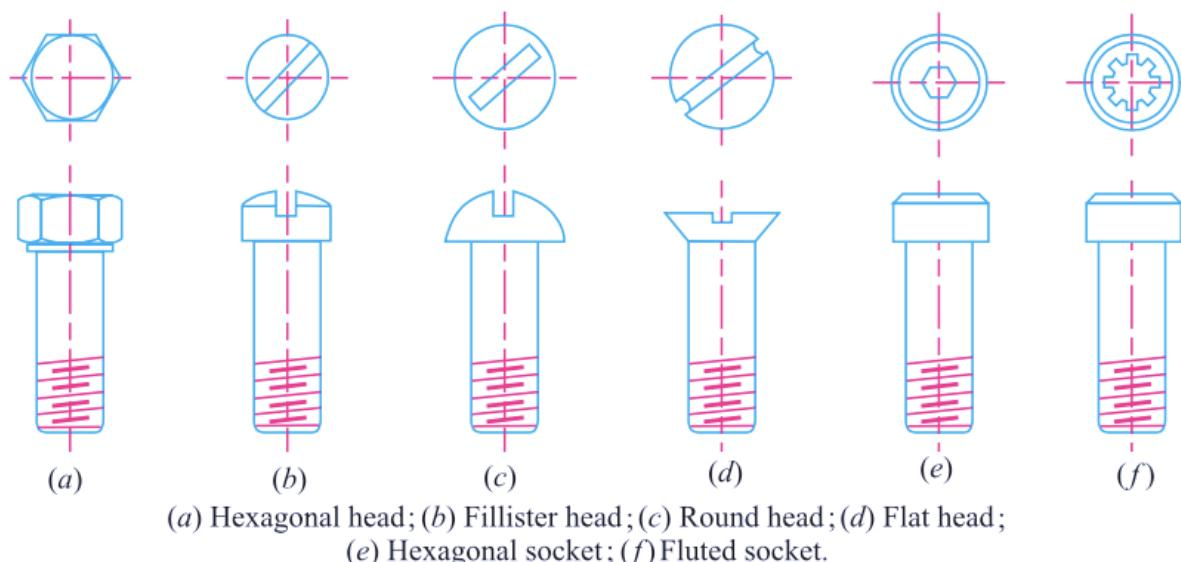
**Fig. 11.13.** Types of cap screws.
