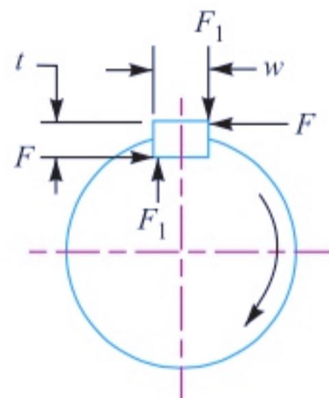
The distribution of the forces along the length of the key is not uniform because the forces are concentrated near the torque-input end. The non-uniformity of distribution is caused by the twisting of the shaft within the hub.
