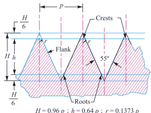
Fig. 11.2. British standard whitworth (B.S.W) thread.
