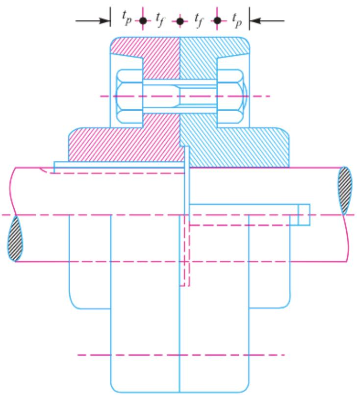
The thickness of the protective circumferential flange ( $t_p$ ) is taken as 0.25 d. The other proportions of the coupling are same as for unprotected type flange coupling.
