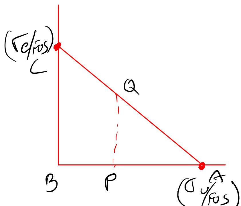
$$\frac{\frac{191 \times 10^3}{d^2}}{\frac{700 \times 10^6}{4}} = 1 - \frac{\frac{446 \times 10^3}{d^2} \times 1.65}{\frac{900 \times 10^6}{3.5}}$$
