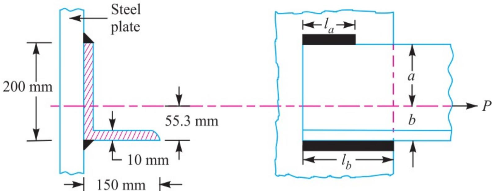
$$P = 200 \text{ kN} \quad \tau = 75 \text{ MPa} \quad l_a = ?$$
