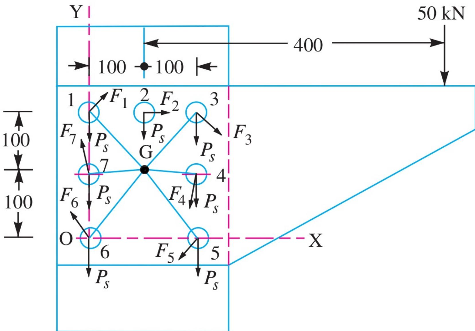
$$P_s \text{ (direct shear)} = \frac{\text{Force}}{\text{no of rivets}} = \frac{50 \times 10^3}{7} = 7143 \text{ N}$$
