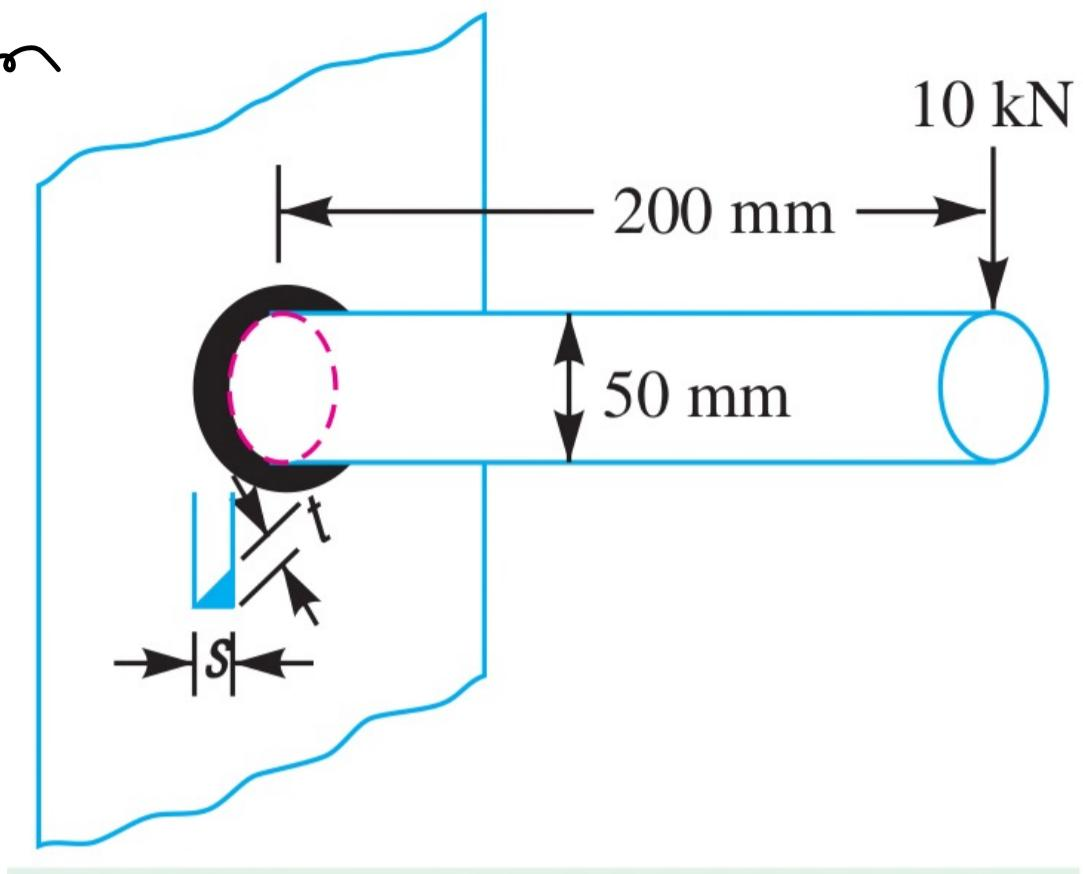
**Example 10.13.** A bracket carrying a load of 15 kN is to be welded as shown in Fig. 10.28. Find the size of weld required if the allowable shear stress is not to exceed 80 MPa.
