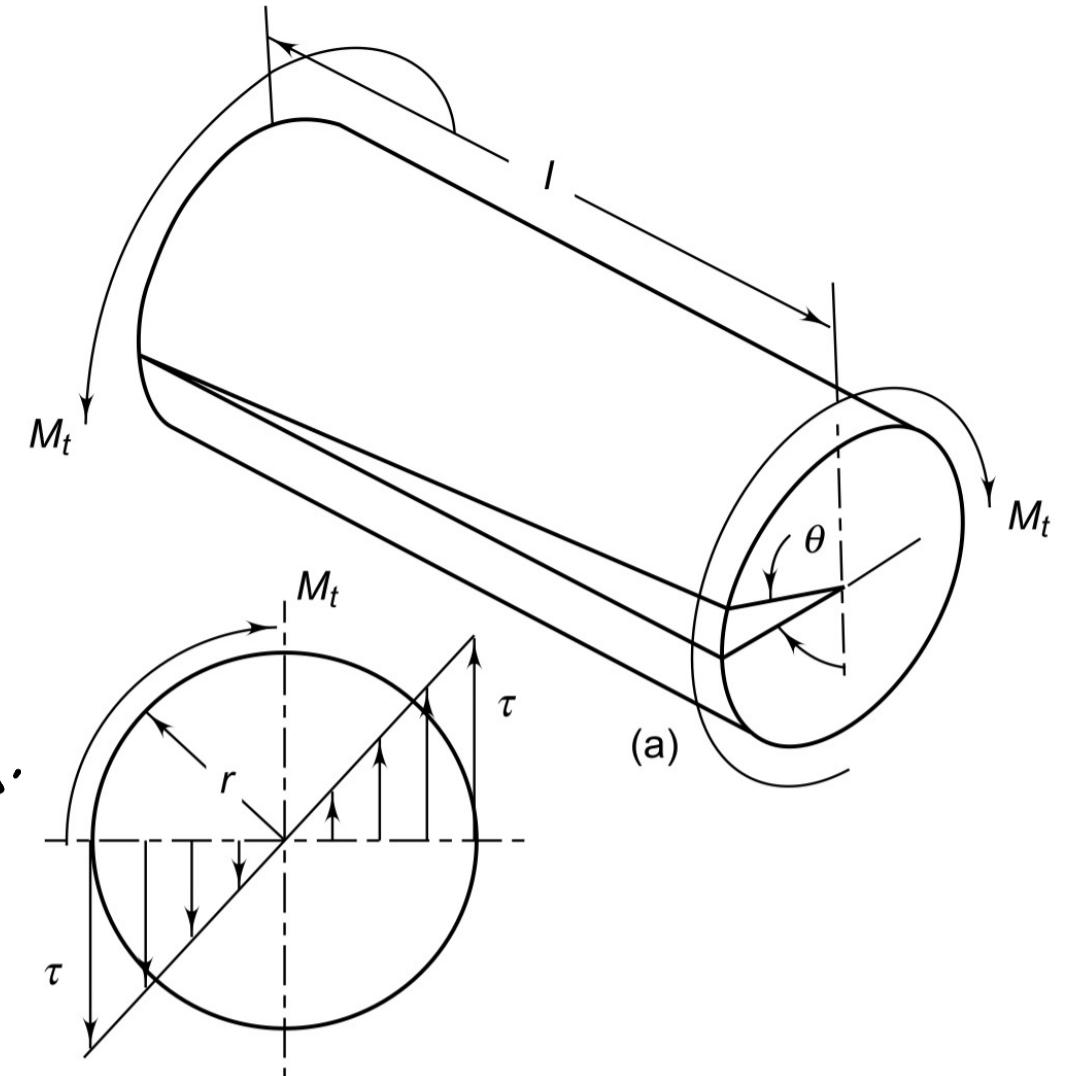
Stress induced due to twisting action (or) moment is called Torsional stresses.
